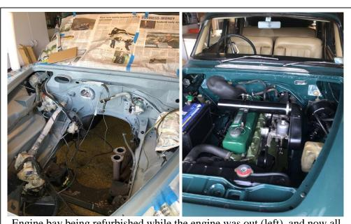
Engine bay being refurbished while the engine was out (left), and now all put back together again, new engine installed.
