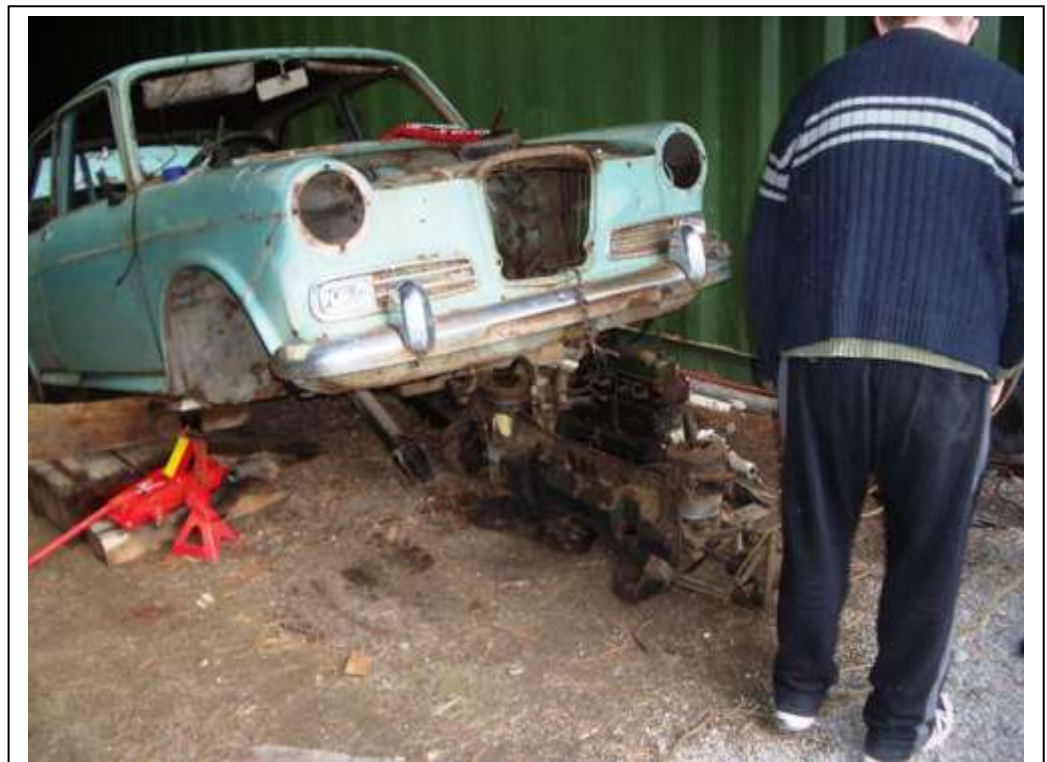
Front sub-frame complete with engine & gearbox is removed from the 1100
