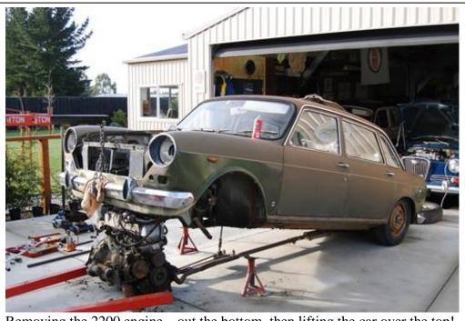
Removing the 2200 engine – out the bottom, then lifting the car over the top!
