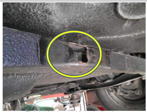
The hole left in the rear subframe after the exhaust mounting bracket broke away on the 1100.
