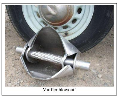
The front half of the exhaust system was new, though it did not sound like it. A look underneath and we found the brand-new muffler was blown wide open and we had not travelled one yard!!
